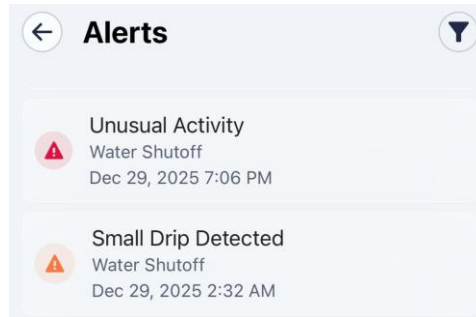
Figure 6. Example of alerts sent by a smart water meter
